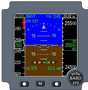
INTEGRATED STANDBY INSTRUMENTS (ISI)
