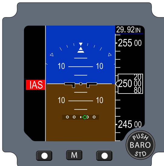
Airspeed failed Figure 08-08-8
