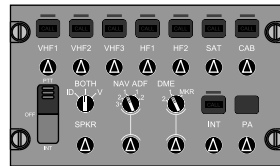
AUDIO CONTROL PANEL (ACP)
