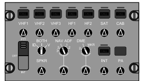
AUDIO CONTROL PANEL (ACP)
