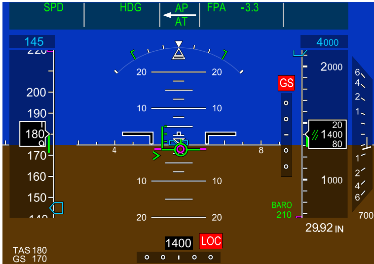
Failure indications Figure 16-01-9
