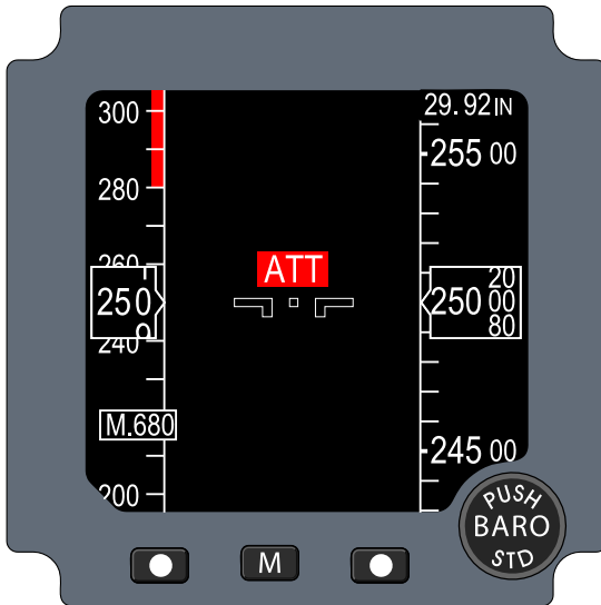
Attitude display failed Figure 08–08–5
