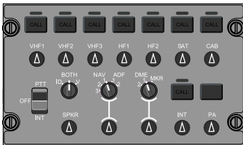
AUDIO CONTROL PANEL (ACP)
